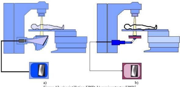
Figure 13: a) scintillation EPID; b) semicontuctor EPID<sup>3</sup>
