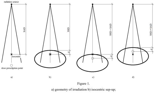
c) fix SSD setu-up; d) mixed mode set-up
